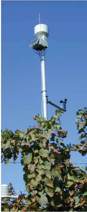
Remote, wireless weather stations collect temperature, relative humidity, precipitation, leaf moisture and solar radiation data at specific sites.
